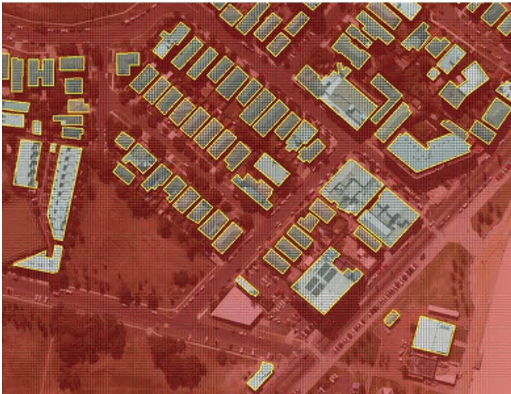
Photo B4: “Nulling” of Grid Cells based on Building Outlines
