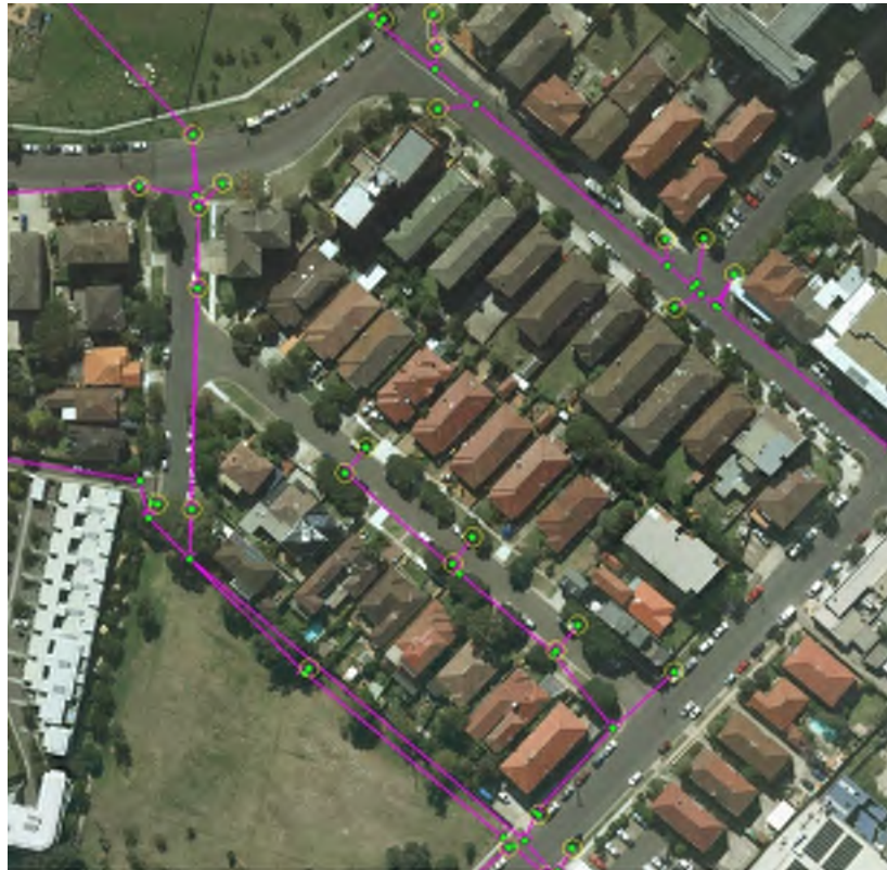
Photo B3: Application of Inflow Boundary Conditions (yellow circles)
