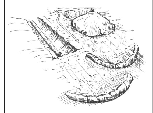
Minimise the width of cut and the time trenches are open - then quickly stabilise the backfill.
