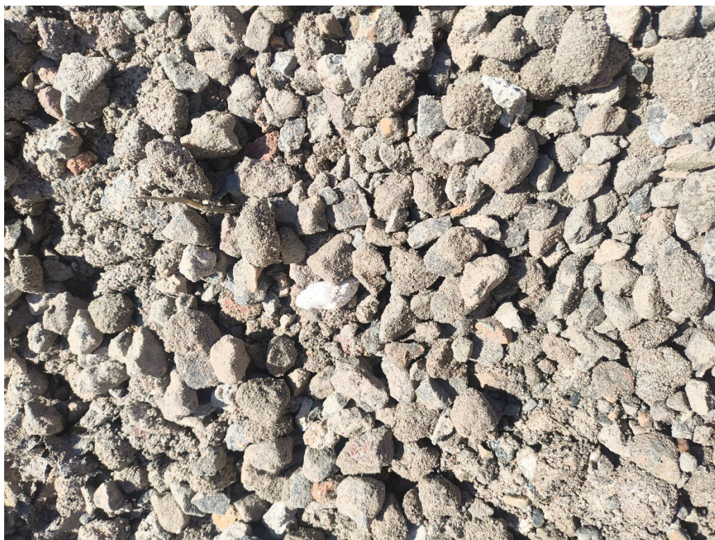
Photograph 2: Recycled DGB20 at source site.
