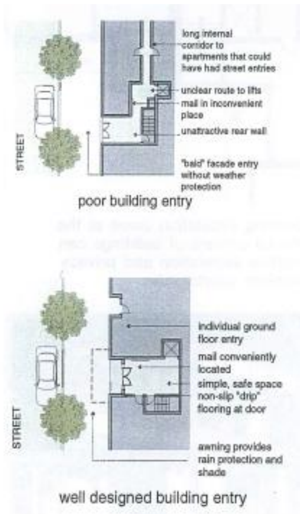
Figure 59: This diagram illustrates a contrast between undesirable practice (top) and better design practice (bottom) for entry and lobby design.
