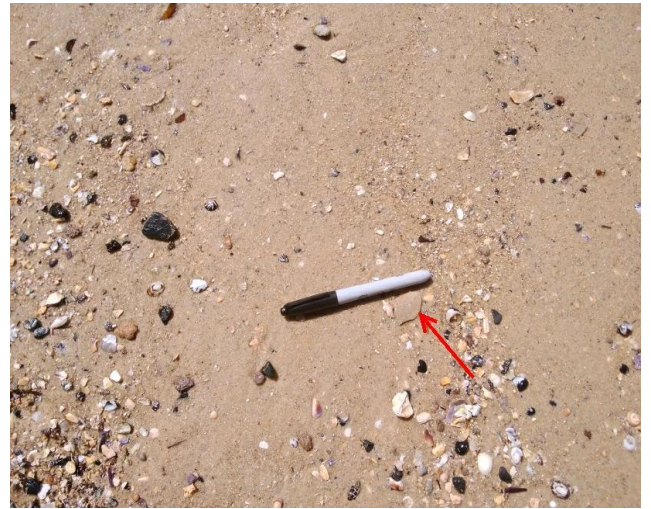
Notes: Overview of the ACM fragment prior to the removal within Northern beach.
