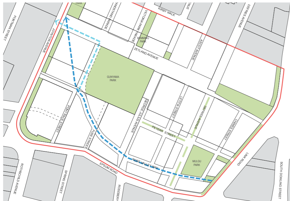
Epsom Park Precinct - Showing trunk drain alignment
