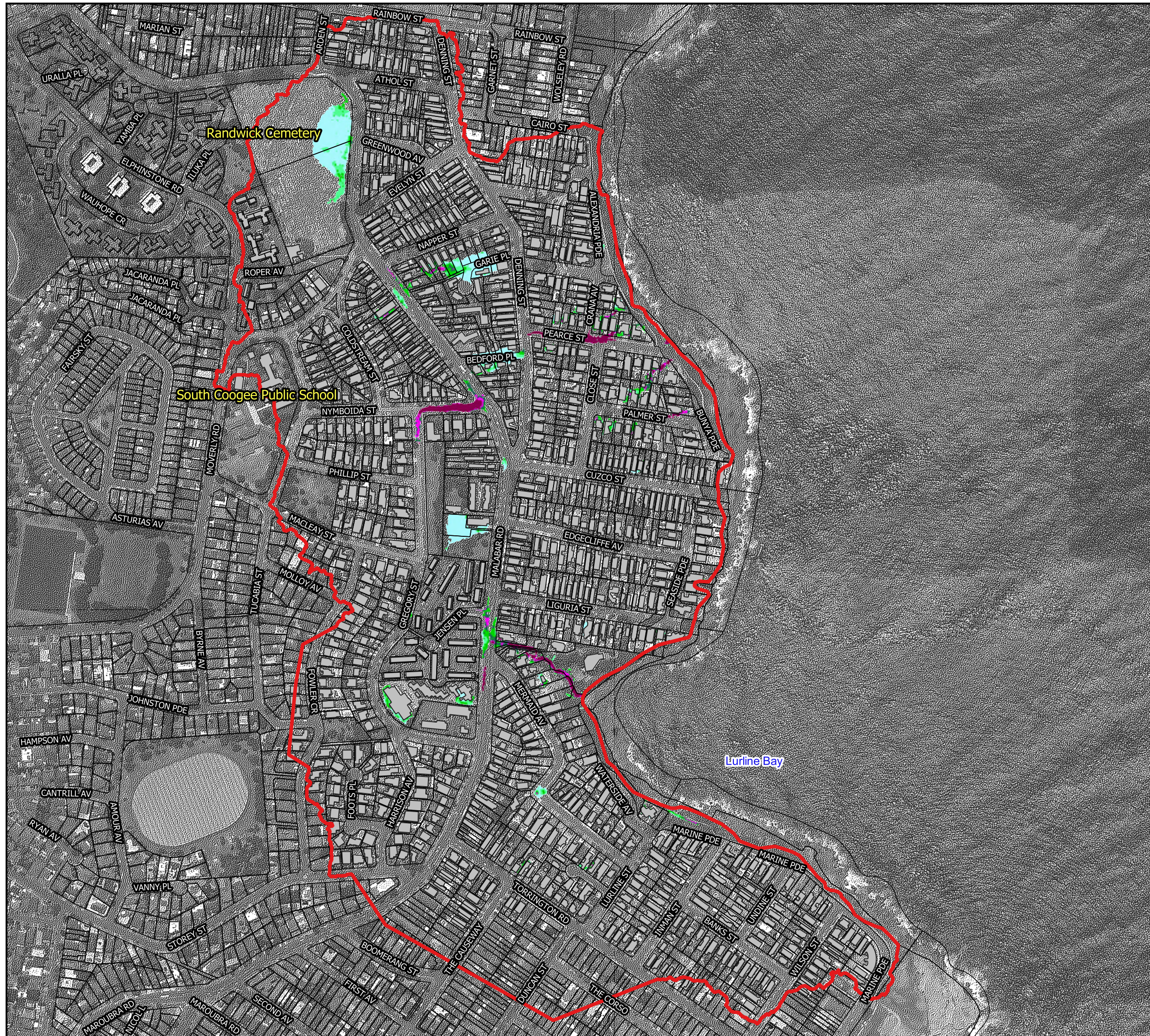
Figure 31.1: Peak Flow Velocity for the 1% AEP Flood
