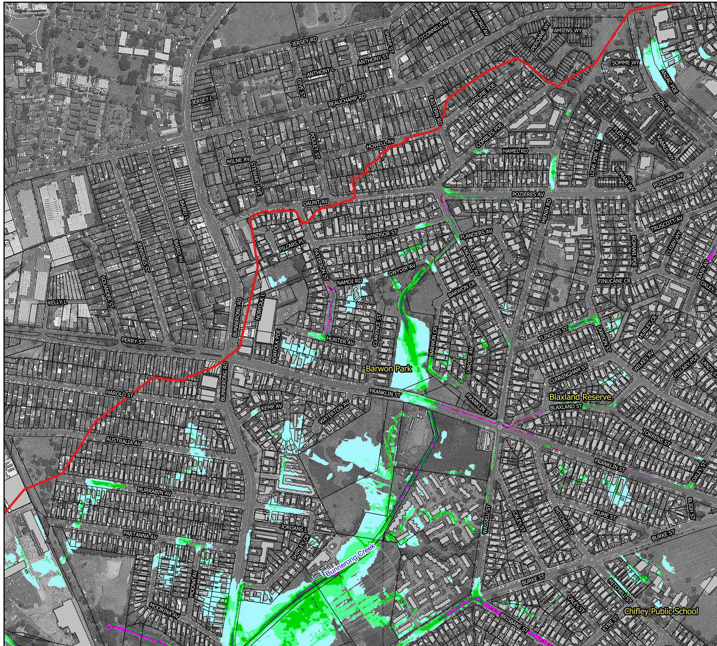
Figure 30.2: Peak Flow Velocity for the 2% AEP Flood
