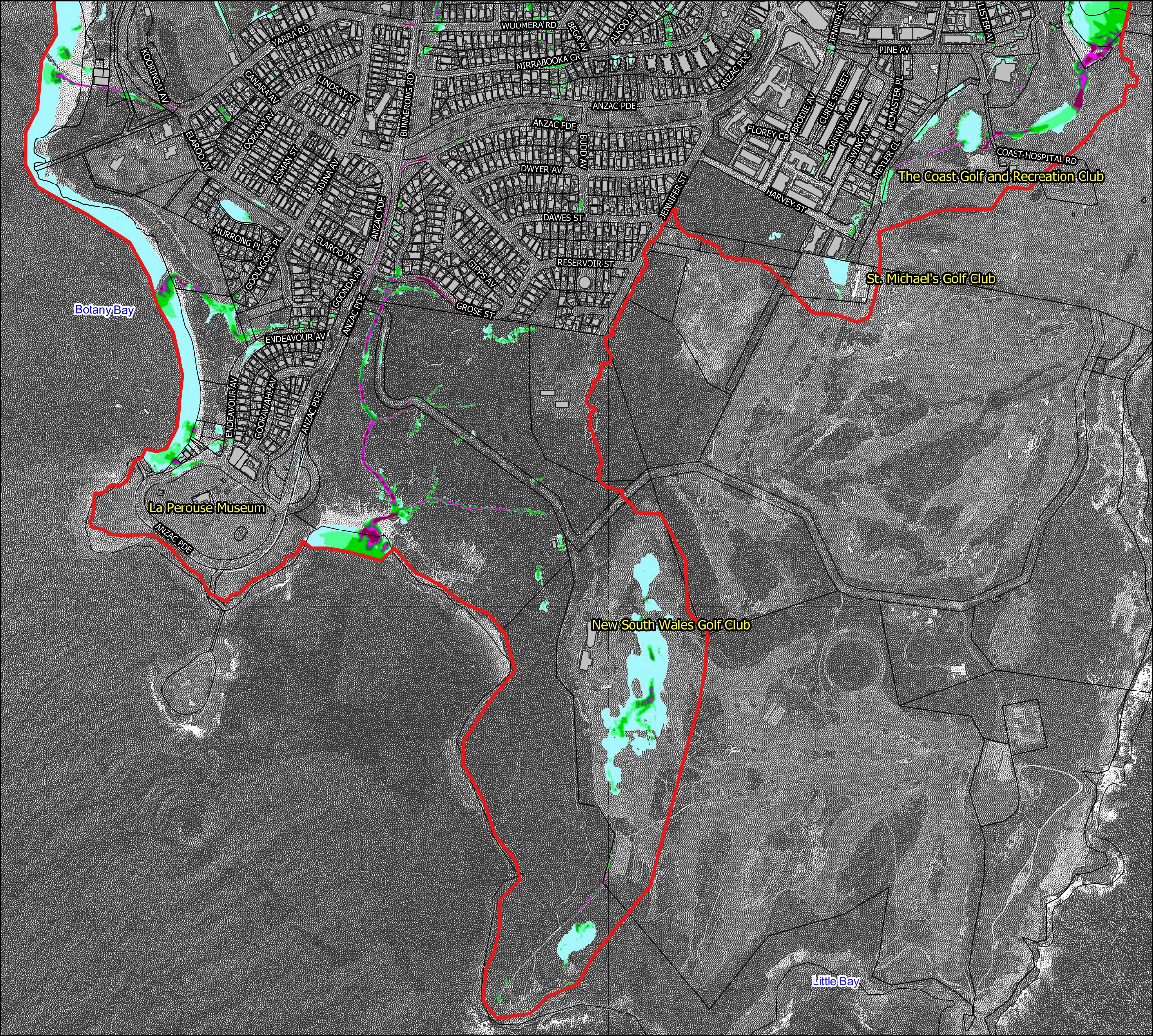
Figure 31.6: Peak Flow Velocity for the 1% AEP Flood
