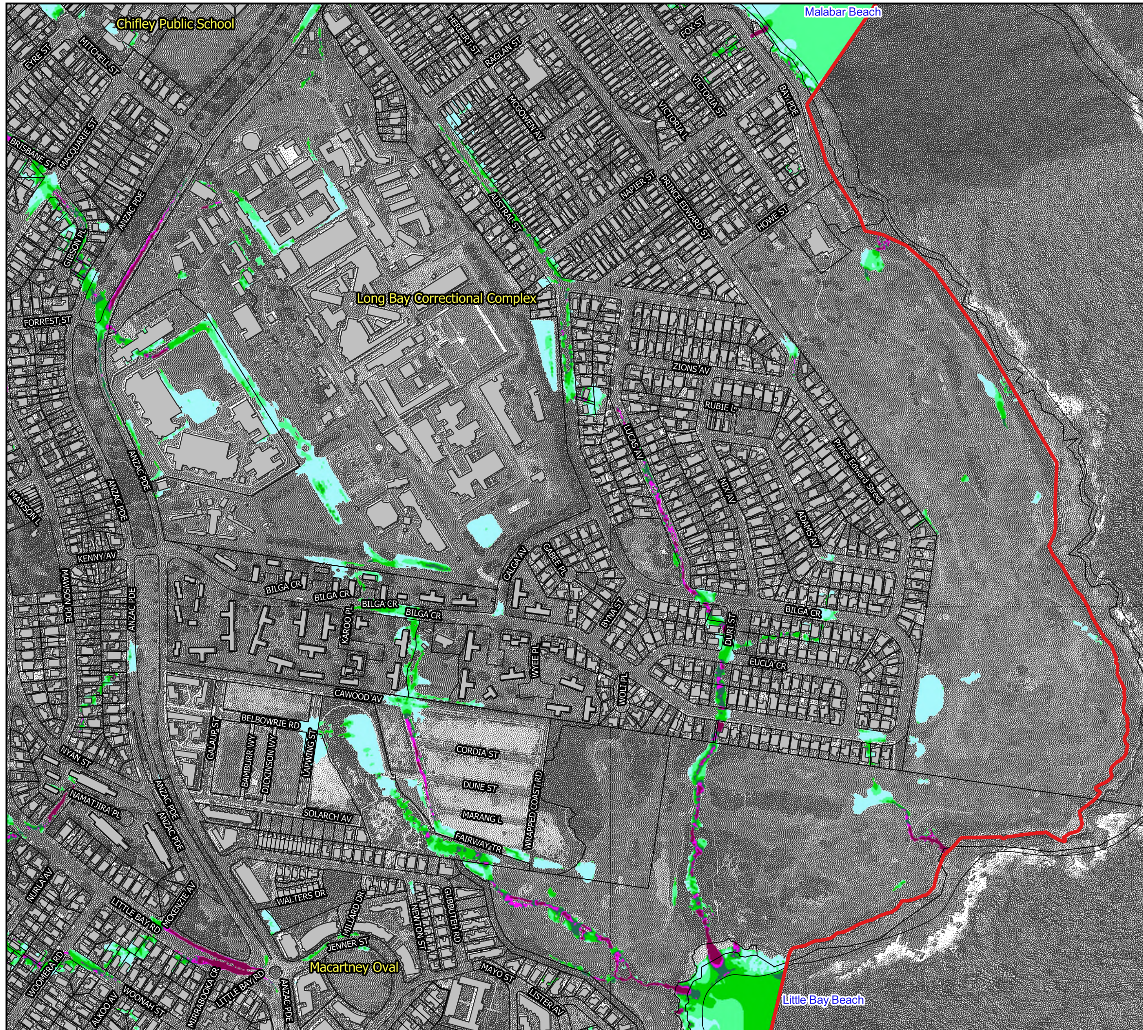
Figure 31.5: Peak Flow Velocity for the 1% AEP Flood
