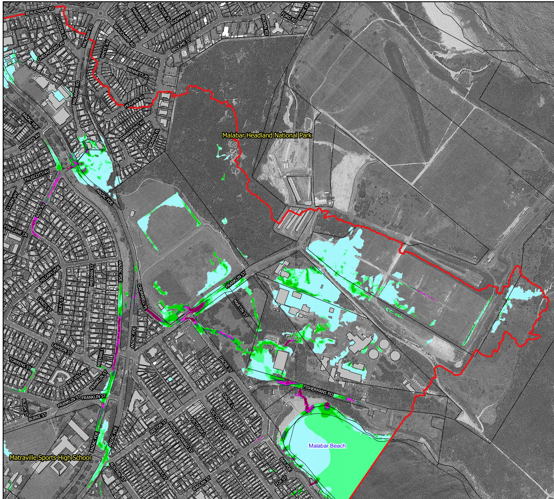
Figure 31.3: Peak Flow Velocity for the 1% AEP Flood
