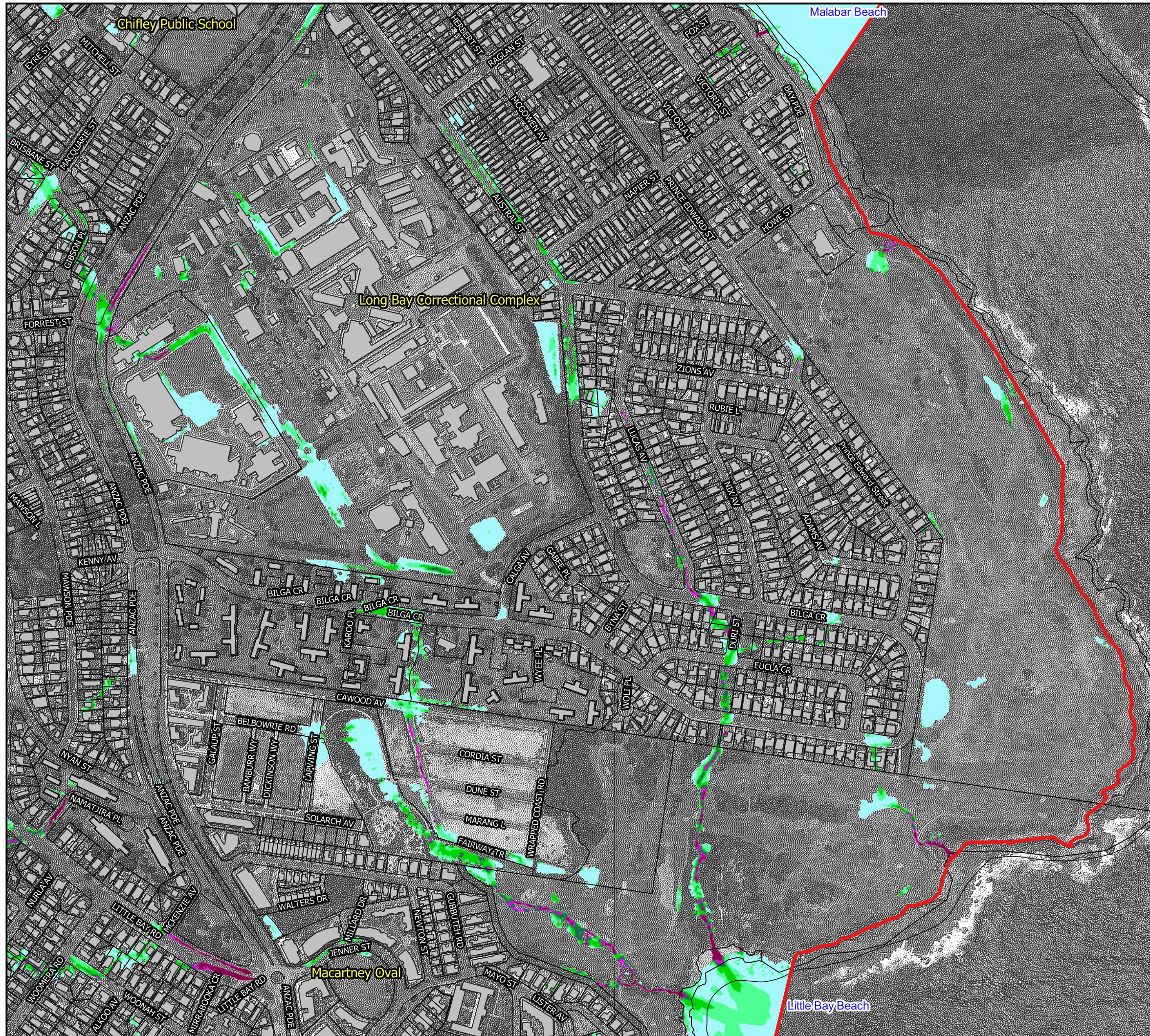
Figure 30.5: Peak Flow Velocity for the 2% AEP Flood
