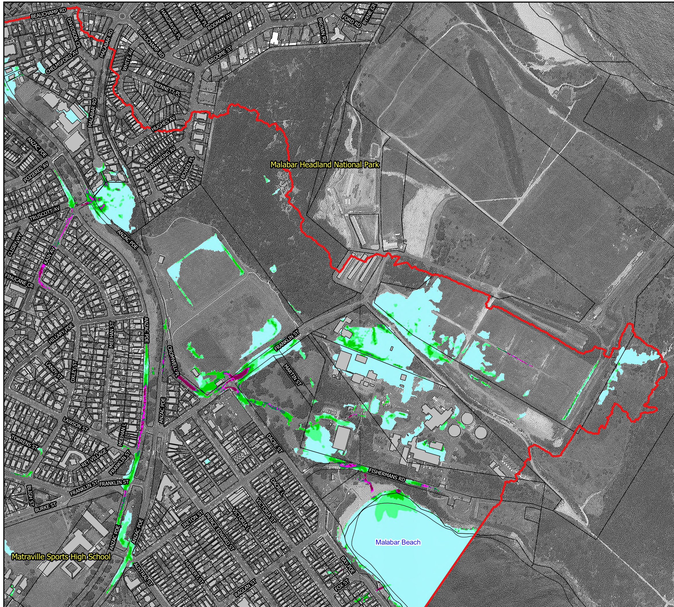
Figure 30.3: Peak Flow Velocity for the 2% AEP Flood
