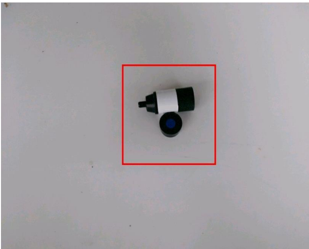
Location: Field Blank Result: 0 fibres / 100 fields Image Id: 230213-150104
