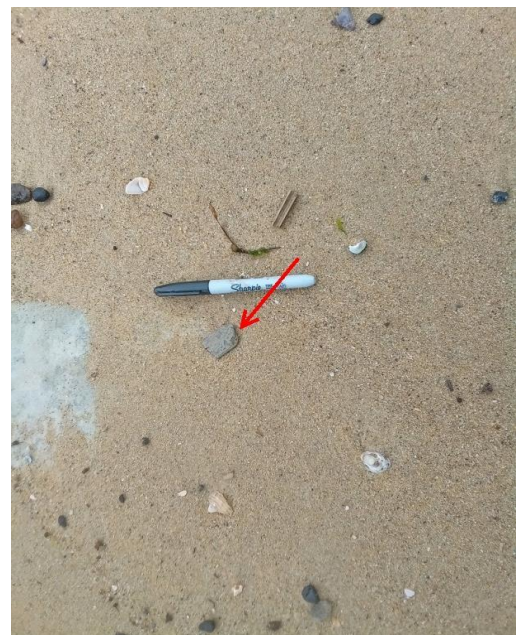
Notes: Overview of the ACM fragment prior to the removal within Northern beach.
