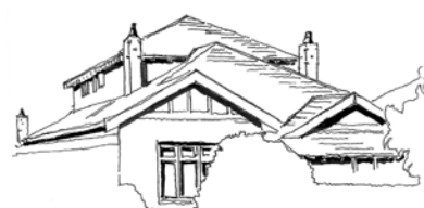
Additions set back from the existing ridgeline retain the form and detail of the existing residences. Use of simple roof forms and subtle detailing further enhances the relationship of new and existing works.
