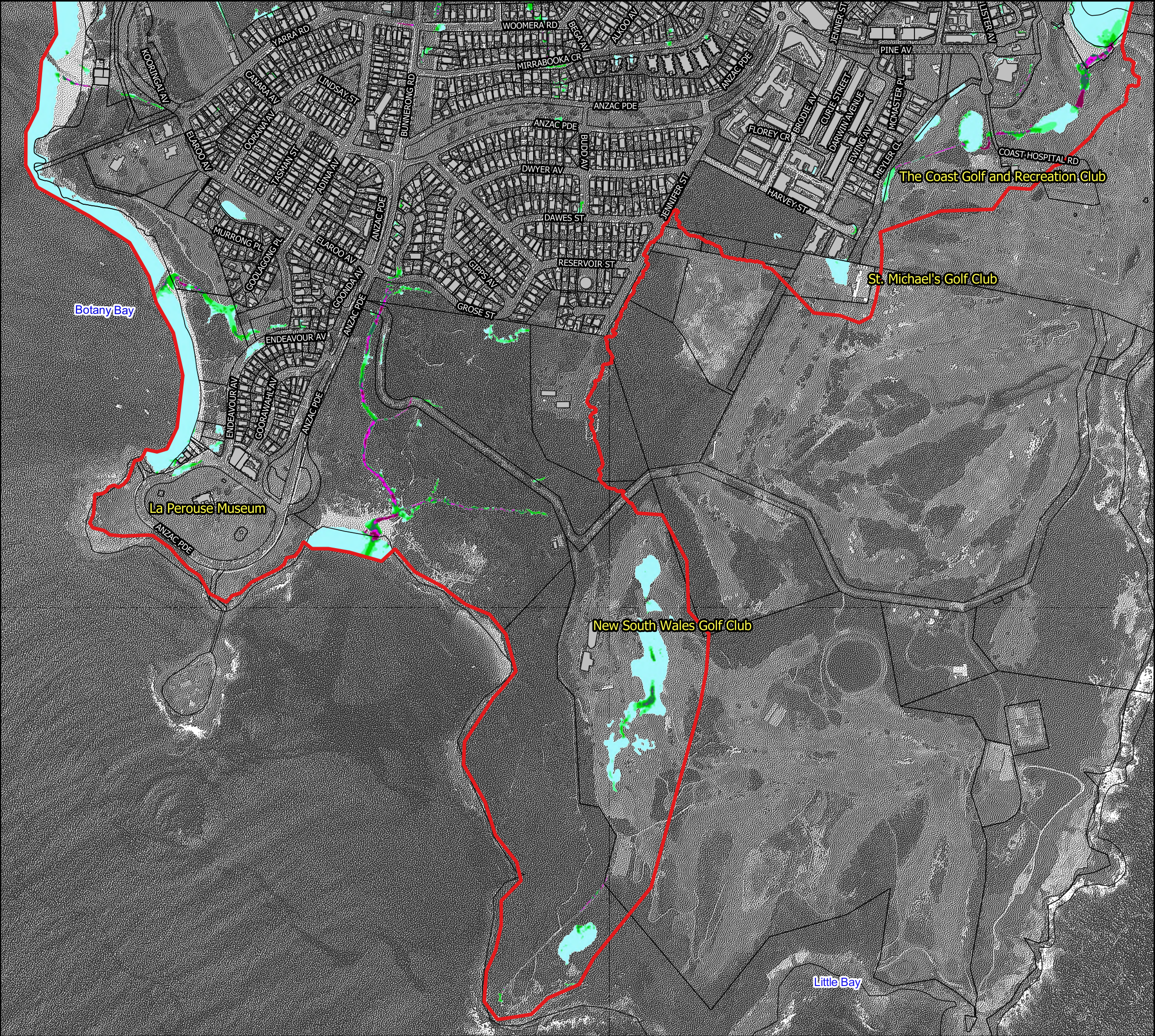
Figure 29.6: Peak Flow Velocity for the 5% AEP Flood
