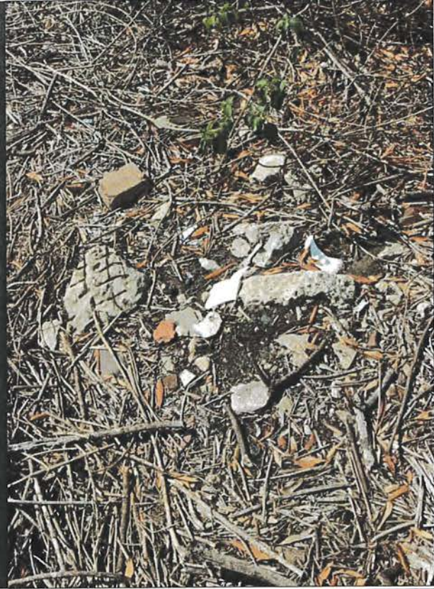
BUILDING WASTE WITH ACM FRAGMENTS
