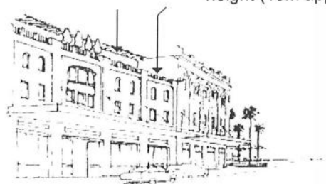
Figure 4 - The development envelope for the site adjoining the Maroubra Bay Hotel includes a 10m street wall height with 12m building height setback 5m from the street alignment.
