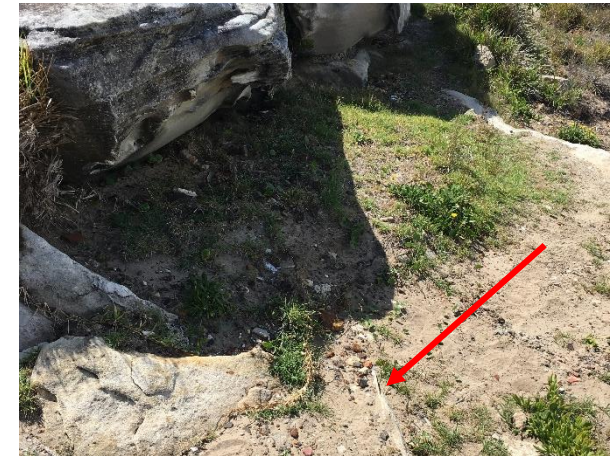
Photo 6: Large compressed asbestos cement sheet partially buried adjacent TP20
