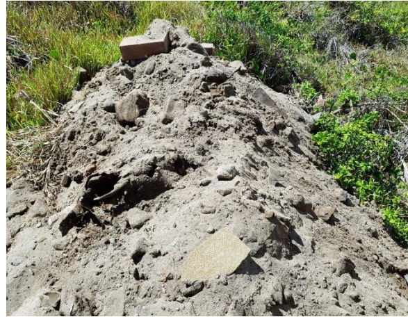
Photo 2: ACM as fibre cement sheet debris and anthropogenic inclusions of brick and concrete in excavated test pit spoil at TP10
