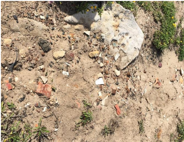
Photo 4: Anthropogenic debris and ACM debris to ground surface at TP19. Surface water run off expected to have resulted in deposits of debris in this location.
