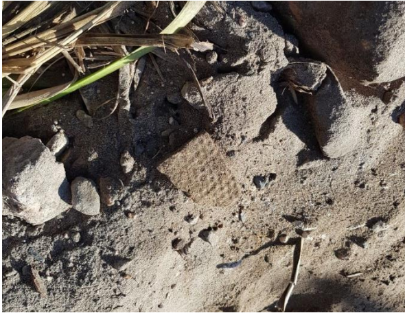
Photo 7: Typical example of ACM debris within sub surface soils (TP04 shown)
