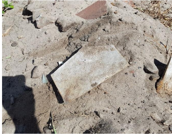
Photo 8: Typical example of ACM debris within sub surface soils (TP10 shown)
