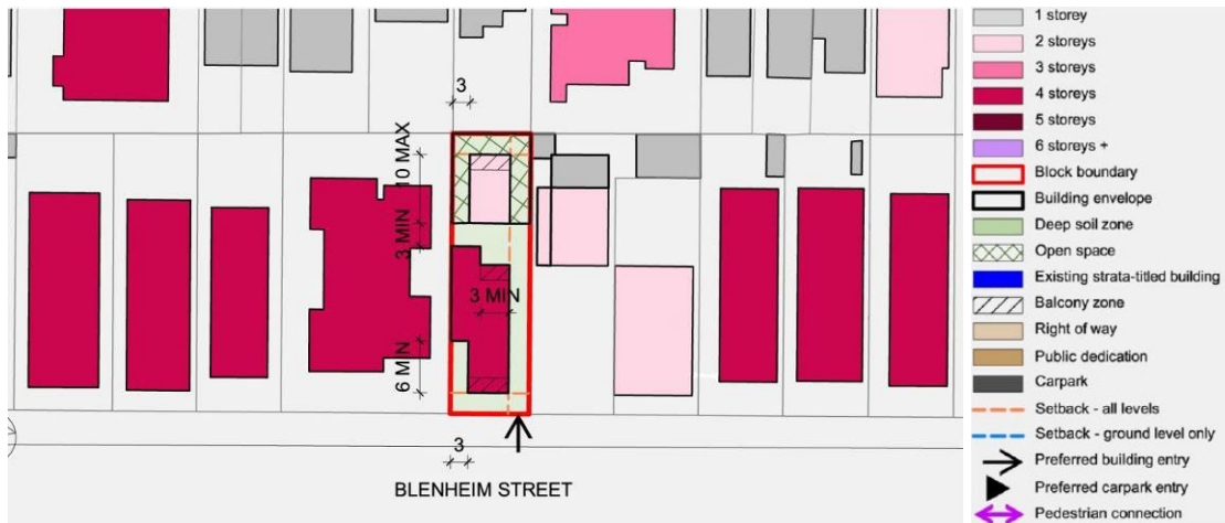
Figure 13: Building envelope - plan
