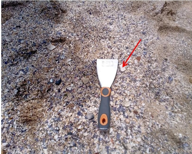
Notes: Overview of the ACM fragment prior to the removal within Southern beach.
