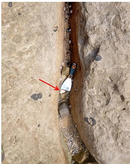
Notes: Overview of the ACM fragment prior to the removal within Northern beach.
