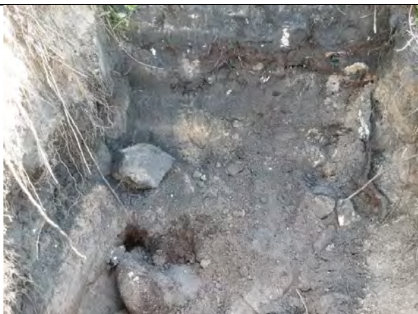
Northern beach, TP05_1.0, Fill with glasses, tiles, brick, plastic, metal, concrete and coal.
