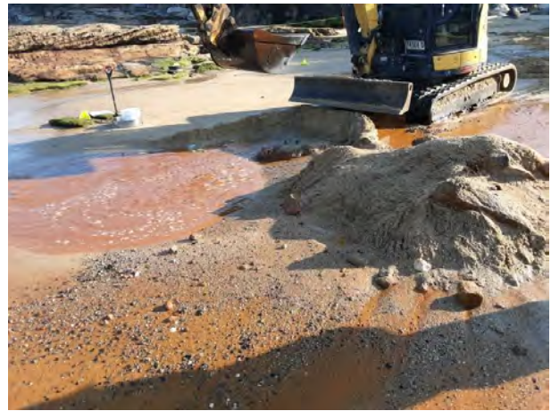
Middle beach, TP29_0.3, Fill with brick, glass, sand, shell, rocks, ACM fragments.
