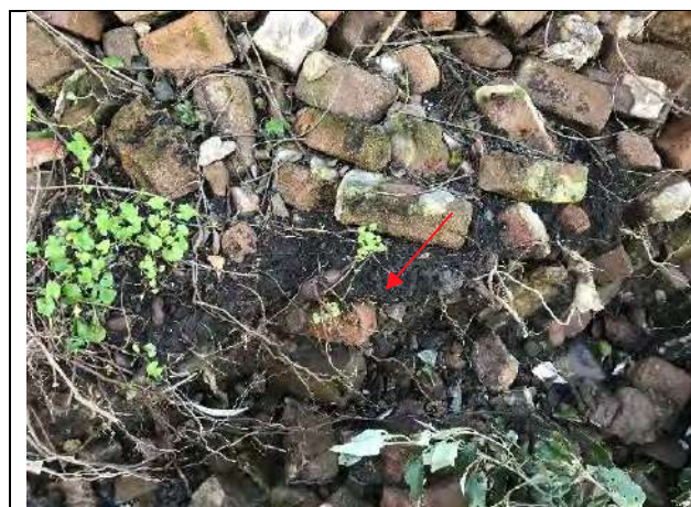
Crown Gully 2, landfill, ACM fragments
