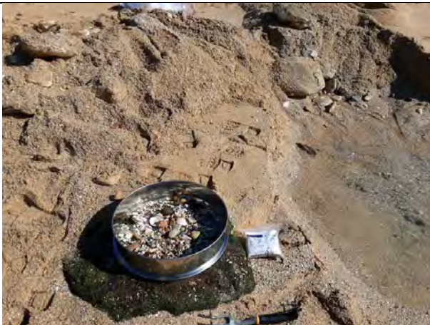
Southern beach, TP41_0.5, Sand and rock with tiles, abundant glasses, fibro cement pieces
