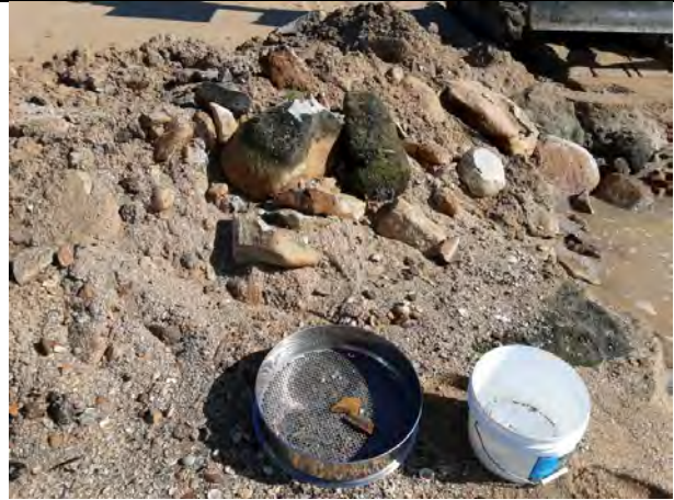
Southern beach, TP41_1.0FC02, Sand and rock with glass, tiles and shell, ACM fragments.
