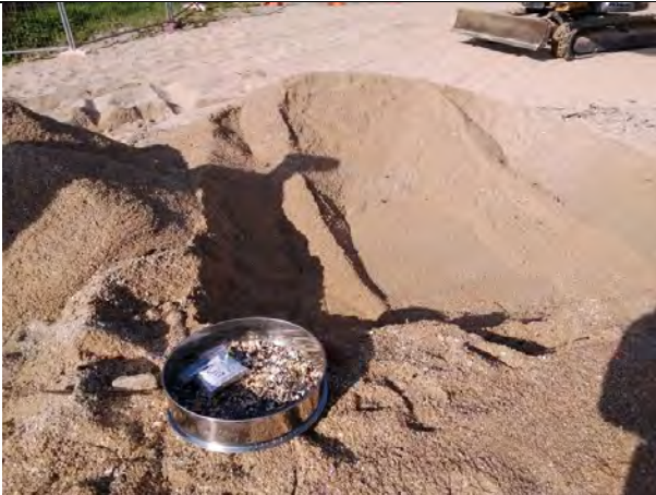
Southern beach, TP36_0.5, sand, small suspected ACM fragment 1 cmx1 cm, sandstone boulders from 0.6 m.
