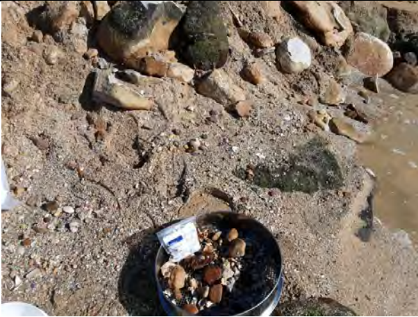
Southern beach, TP41_1.0, Sand and rock with glass, tiles and shell, ACM fragments.
