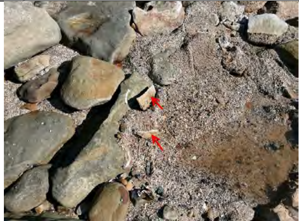
Southern beach, TP39_0.1, Rock and sand with FC sheeting fragments 1.5 kg.
