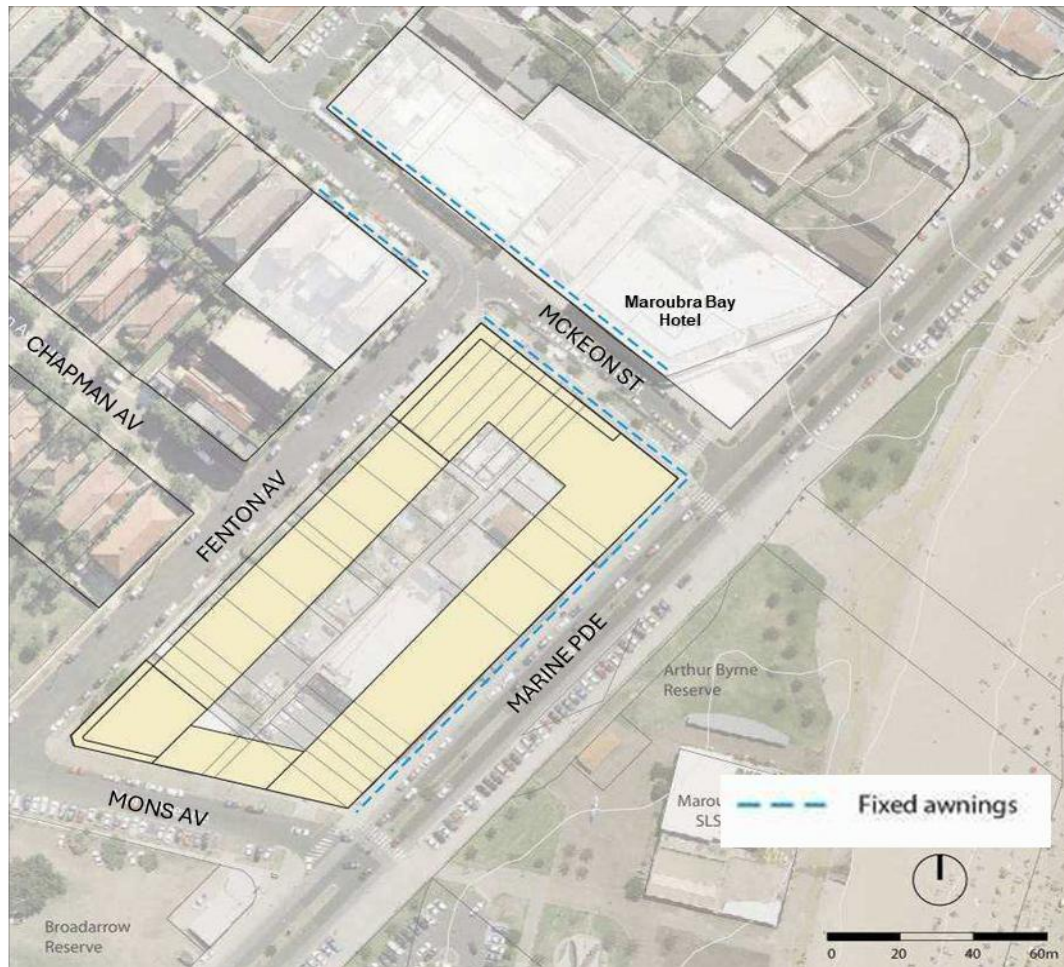
Figure 14: Awnings base scheme
