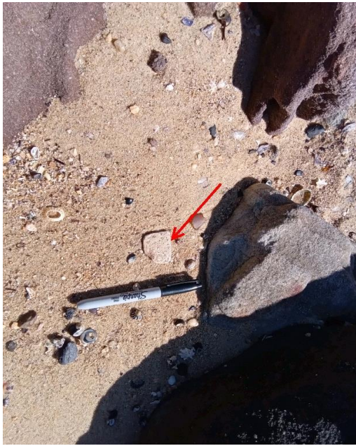
Notes: Overview of FC fragment within Northern Beach prior to the removal.
