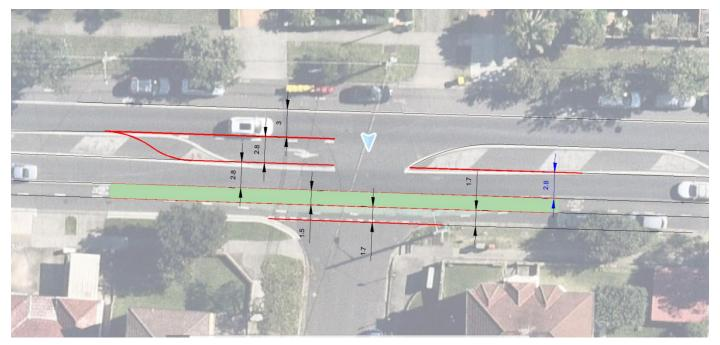
The design seeks to realign the cycleway northerly along Edgecliff Road and straighten the alignment to match the existing road widths (currently 2.8m upon approach of the intersection labelled by the blue dimension). This will allow a greater buffer and provide better sightlines leading for vehicles within the Malabar Road and Edgecliffe Avenue intersection. The Concept Plan is currently being reviewed and once finalised will be tabled at an upcoming Traffic Committee meeting.
