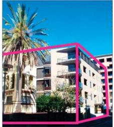
A building envelope is NOT a building. It is the maximum three dimensional shape within which a building will be designed.
