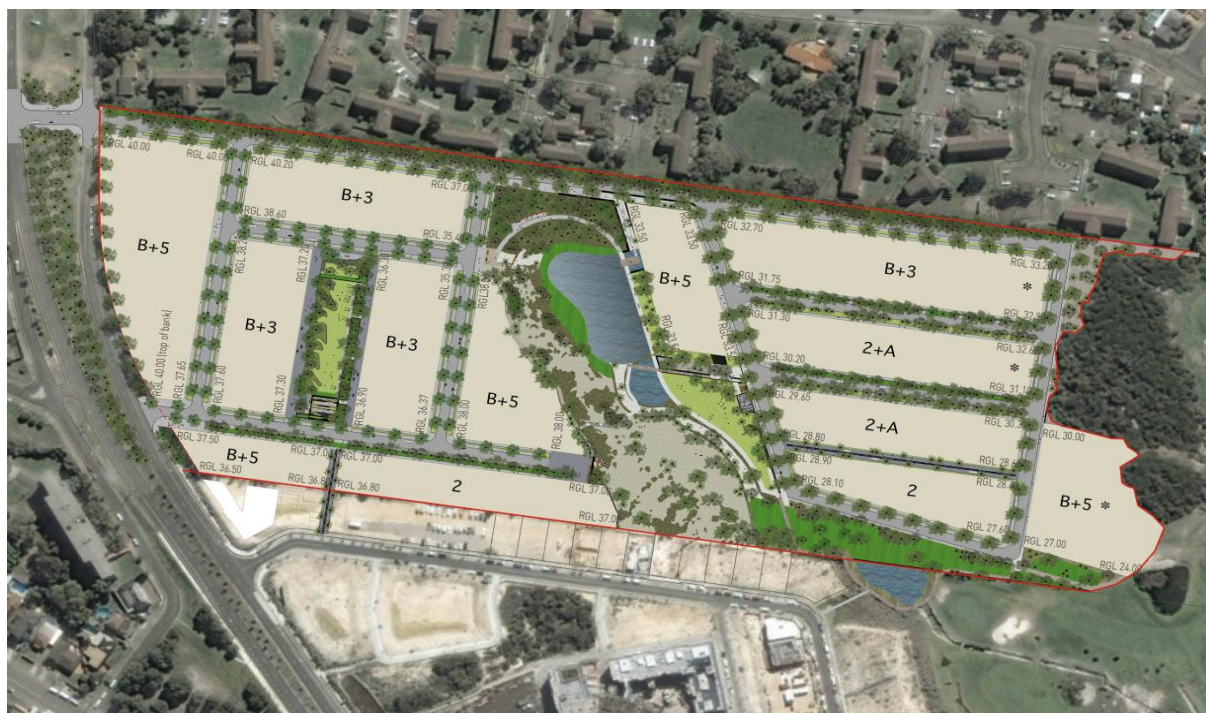
Figure 22: Building height control plan
