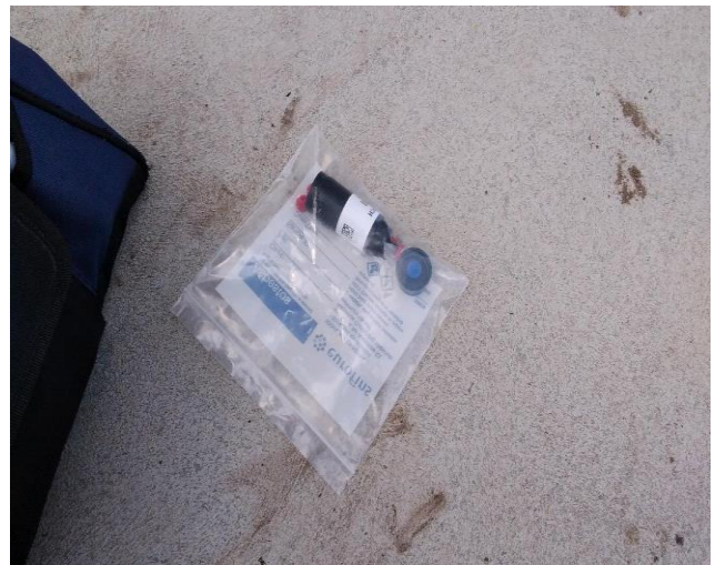
Location: Field blank Result: 0 fibres / 100 fields Image Id: 230603-122121
