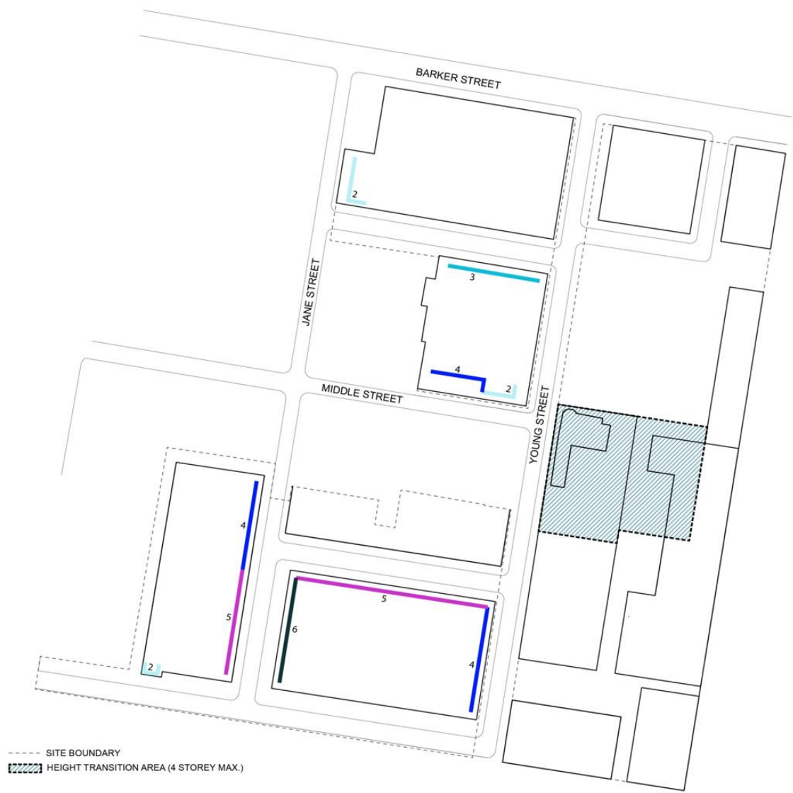
Figure 11: Indicative building edge heights in key areas
