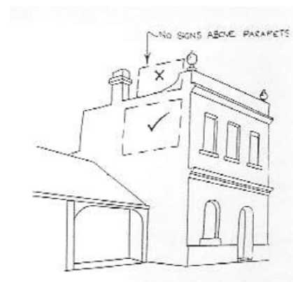
No signs above parapet
