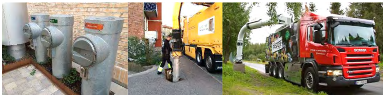
Figure 3-2 - Local Collection System Using a Mobile Vacuum Collection Vehicle and Docking Point
