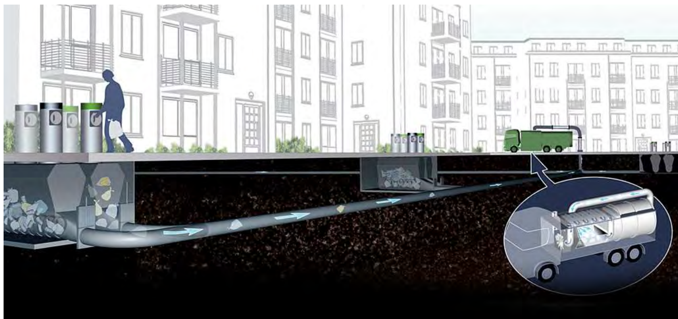
Figure 3-1 - Schematic of Local Collection System Underground Tanks and Mobile Vacuum Truck
