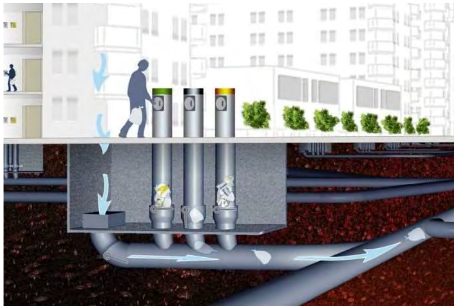
Figure 3-5 - On Street Inlets Schematic
