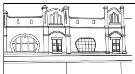
Examples of parapet roof forms
